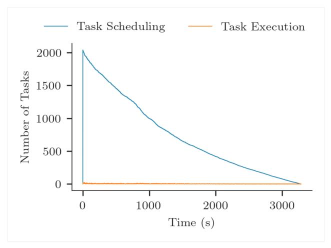
The plot above shows that tasks are between 'AGENT\_SCHEDULING' and 'schedule\_ok' at the beginning of the execution (dark blue). Few seconds later, tasks start to be between 'rank\_start' and 'rank\_stop', i.e., they are scheduled and start executing. Tasks appear to have a relatively heterogeneous duration, consistent with the task runtime distribution measured in *duration analysis*.
